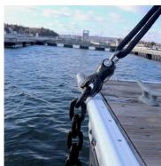
Designed with a 4:1 safety factor, SEA-Snap™ instantly takes hold and will not release under load. For highly dynamic or long-term connections SEA-Snap™ has an integrated locking pin to protect against accidental disconnection. Disconnection is a simple one-handed operation, making SEA-Snap™ an obvious choice for diver and back-deck operations.
